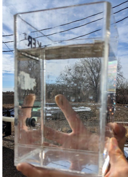
Figure 2 – Filter effluent water. The calibrated turbidity analyzer was indicating in the 0.050 NTU range.
