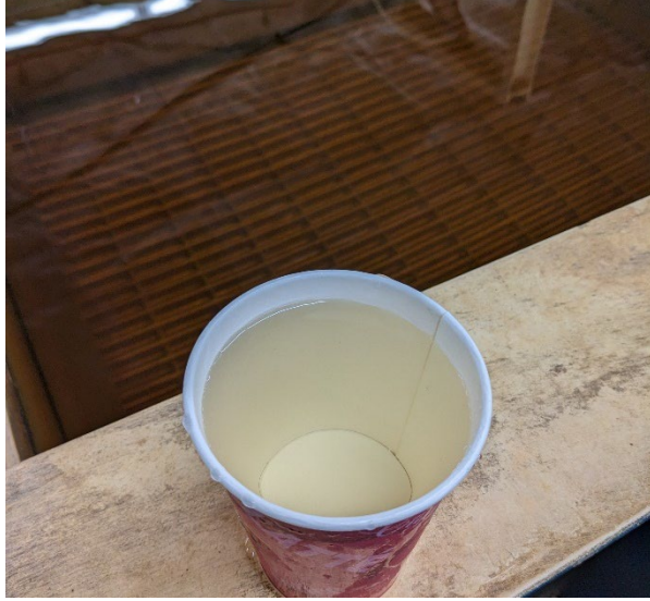
Figure 1 – Top of filter water after increasing permanganate additions. A spot check at 2 ppm permanganate was 4 NTU turbidity.
